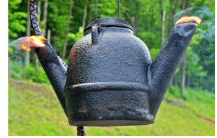
A “Yellow Dog” - an early type of lantern used to illuminate oil derricks
