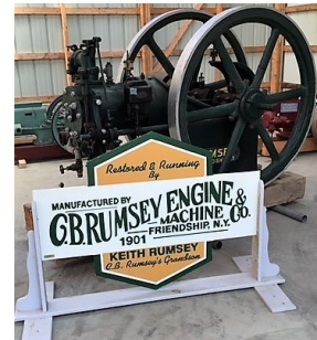
One of the Rumsey engines; this piece is 12 HP and ran equipment in the oil fields
